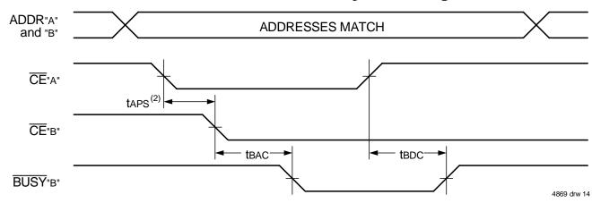
Waveform of **BUSY** Arbitration Cycle Controlled by Address Match Timing  $(M/\overline{S} = VIH)^{(1)}$
